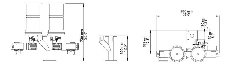
Figure 2. "Duo" Dual Station Digital Dosing Feeder
